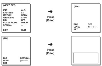
For items in the BLC menu, the user can set the size and location of the BLC area by pressing [ENTER] key after put the cursor on USER... using the [Left, Right] key. For SIZE items, you can use the [Up, Down, Left, Right] key to designate the SIZE, and then press the [ENTER] key. You can set the location for areas using the [Up, Down, Left, Right] key in the LOCATION.
